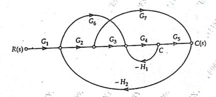
(B) Represent the following system in state space in phase variable form and draw its state model.
